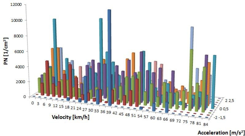
Fig. 15. Emission of PN in the range of vehicle speed and acceleration during economic drive
