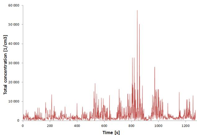
Fig. 6. Total concentration of PM during dynamic drive
