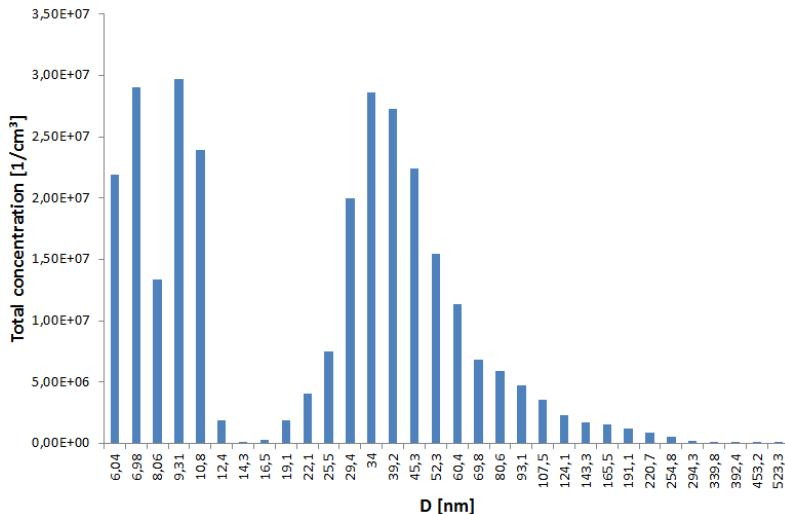
Fig. 8. Dimensional distribution of PN during dynamic drive
